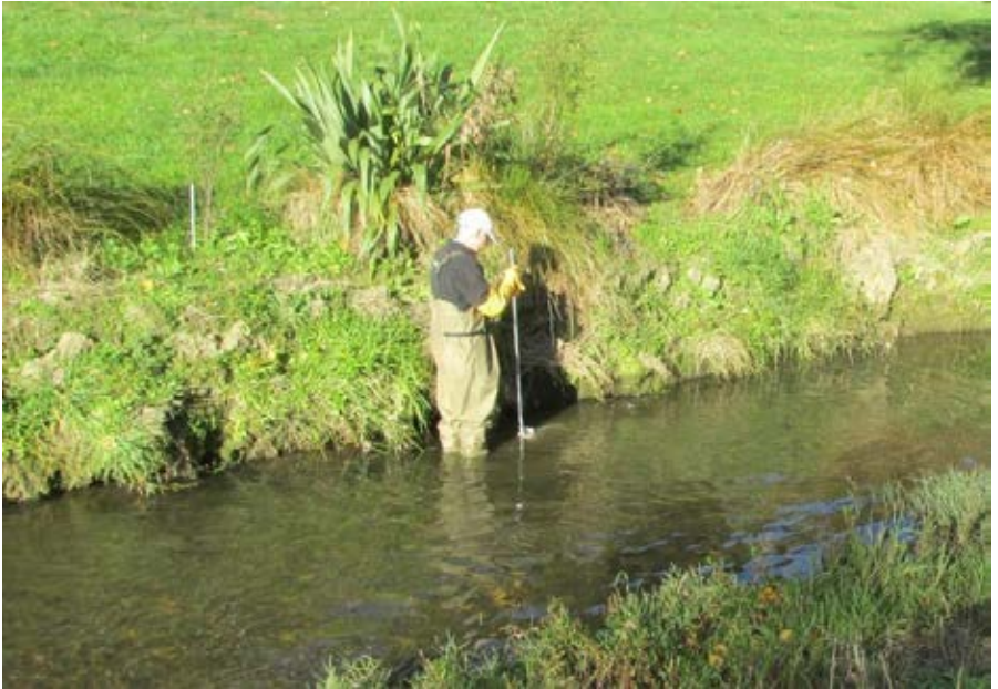
Fig. 7: Obtaining a kick sample by disturbing the streambed in the run section
