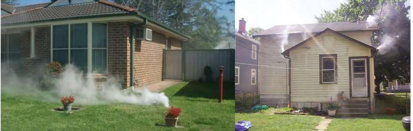
The left picture shows a smoke test detecting a broken pipe, with smoke escaping from the break. The right picture shows a cross connection, where the stormwater collected from the house is being piped to a sewerage pipe.
